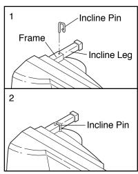
left side. Remove the incline pin from the right incline leg as shown in drawing 1. Adjust the incline leg to the desired height and fully re-insert the incline pin. Make sure the incline pin is in the "locked" position shown in drawing 2. Lay the treadmill on its right side. Repeat the procedure for the left incline leg.
